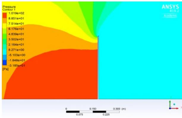
**Figure 2:** Solid Fence pressure profile
