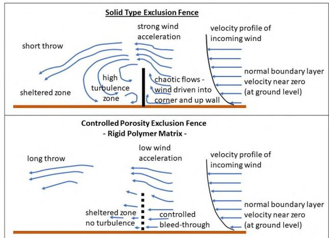
**Figure 8:** Flow profile comparison: Solid vs. Porous (50% Open Area) Exclusion Fences
