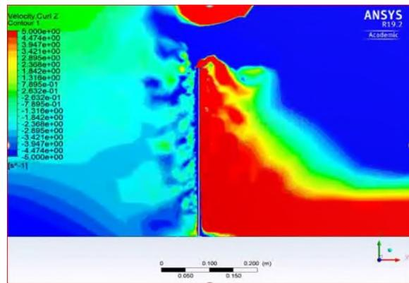
**Figure 4:** Solid Fence vorticity: indicates chaotic/turbulent swirling flows in both directions on both sides of the fence.
