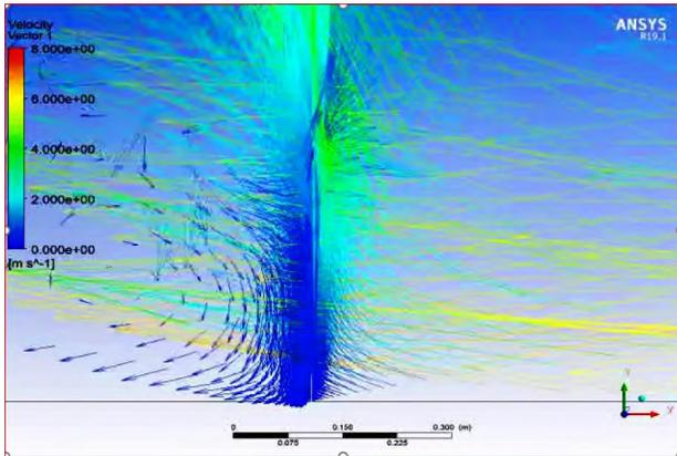
**Figure 7:** Velocity vector analysis: Solid Fence
