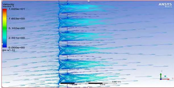
**Figure 6:** Velocity vector analysis: Porous Fence – a zoomed-in view of flow thru the open pores showing rapid dissipation on downstream side (50% open area)
