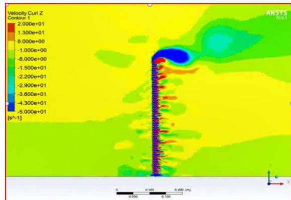
**Figure 5:** Porous Fence vorticity: except within the pores, this graph indicates flows are much like having no fence at all.
