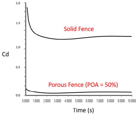
**Figure 1:** Coefficient of Drag in steady state at 5 meters/second. Porous vs. Solid Exclusion Fence
