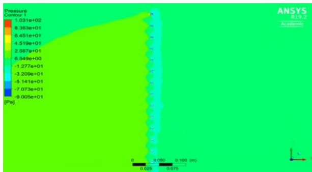
**Figure 3:** Porous Fence pressure profile
