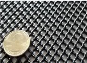
Photo 1: E-Fence™ HDPE Polymer Matrix
